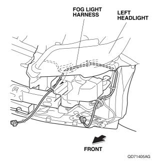
36. Route the fog light harness along the bumper beam. Secure the clip on the fog light harness to the bumper beam as shown.
