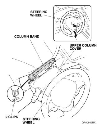
2. Press the engine switch to ON. Turn the steering wheel 90° clockwise. Using a plastic trim tool, release the lock as shown.
