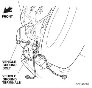
31. Locate the vehicle 1-pin connector taped to the vehicle harness. Remove the tape to free the vehicle 1-pin connector.
