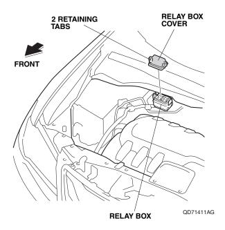
43. Install the relay into the relay box.
