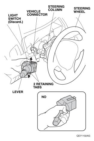
Push in two retaining tabs, slide the light switch, and remove it from the steering column.
